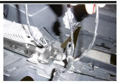
Note: Air vent may need to be trimmed to remove possibility of rubbing through the wiring.
